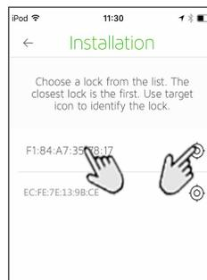
**Note:** You can tag modules in the list by tapping the cross-hair pointer. The LED on the bottom of the module flashes.
