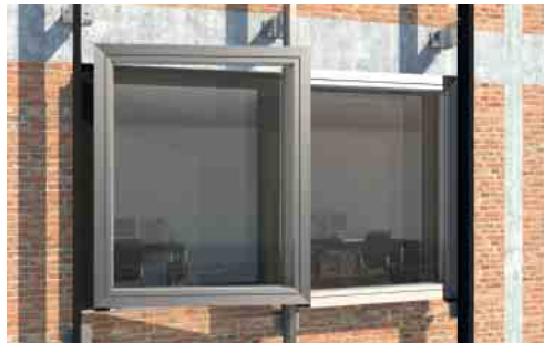
3. Fenstereinbau an die Lisene 3. Installation of windows on the plaster strips
